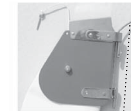
figure 76 | rudder downhaul line
